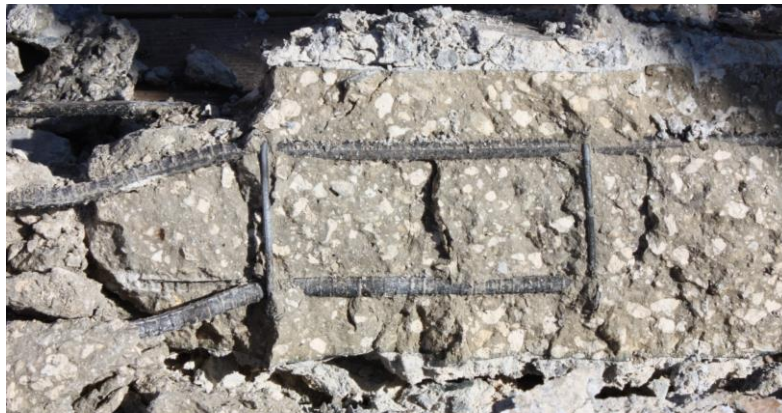
Figure 14. Corrosion-free steel in much of Bridge C submerged region. Note that pile in photo was lying on its side.
