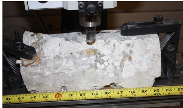
Figure 22. Concrete fragment mounted on mill table. (Bridge B) Note that the measurement datum for the indicated depth was the waterline of the in-service pile.
