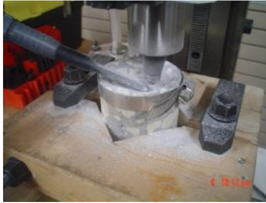
Figure C6. Core mounted on mill table.
